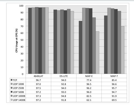
Figure 4 CPU Usage x Packet Size x Technique
